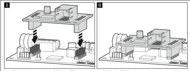
Fig. 8. Installing the GSM-X-ETH module on GSM-X LTE module electronics board.
