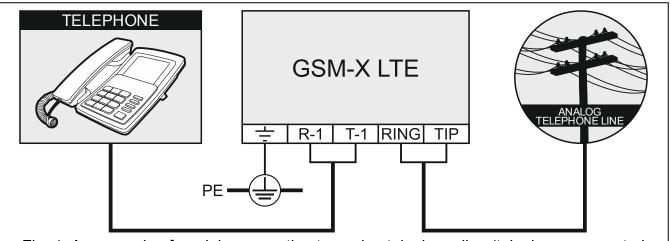
Fig. 4. An example of module connection to analog telephone line (telephone connected to the module).
