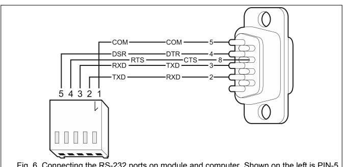
Fig. 6. Connecting the RS-232 ports on module and computer. Shown on the left is PIN-5 plug. Shown on the right is DB-9 female connector (solder side view).
